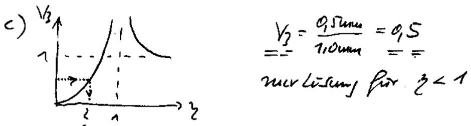
$$V_z = \frac{z^2}{1-z^2} \Rightarrow V_z - V_z z^2 = z^2 \Rightarrow V_z = z^2(1+V_z) \Rightarrow z = \sqrt{\frac{V_z}{1+V_z}}$$
